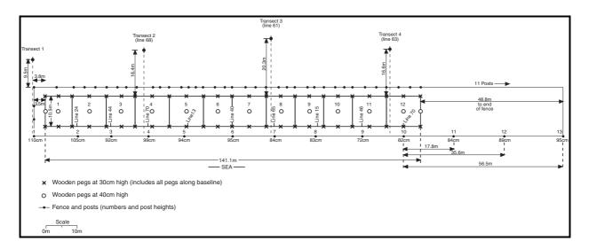
Figure 9: Location of transects and pegs for monitoring changes in sand level on a reshaped foredune, Oakura Beach, New Plymouth.
