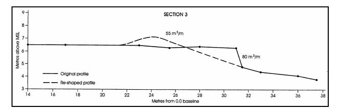
Figure 3: The aim with reshaping the dune at Oakura Beach was to change the original steep foredune profile to an approximately 18° slope extending 10 m wide on which a dense cover of native sand-binding species could be established (from Hesp and Grant 2000).
