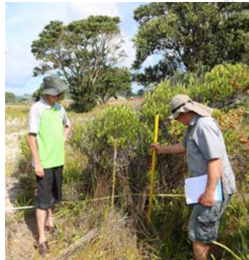
A rapid point sampling method using a transect set up across the dune perpendicular to the coast.
